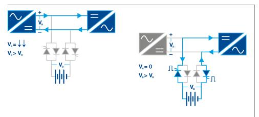
When battery is charged and mains are stable, it is protected from the DC-link ripple by a Green Conversion solid state dynamic battery switch, acting as a digital filter eliminating the chief cause of battery ageing. Green Conversion inverter control enhances system efficiency by reducing IGBTs commutation losses. During mains outages Green Conversion controls the dynamic battery switch SCRs and the battery feeds the inverter.
