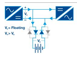
Battery is charged controlling the dynamic battery switch diodes on an intermittent basis, as per battery manufacturers recommendations, or after a discharge has occurred.
