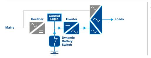
Ultra High Efficiency on-line mode: the inverter feeds power to critical loads whenever mains quality is outside tolerance limits.
