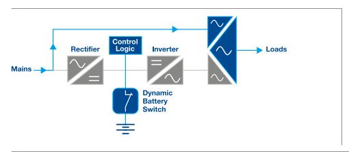
Ultra High Efficiency normal mode of operation: UHE control logic protects critical loads by monitoring power mains quality, while feeding them via the static bypass line.
