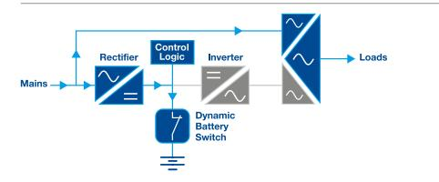
Ultra High Efficiency interactive mode: if input mains stability and reliability is outside preset limits, Ultra High Efficiency interactive mode of operation is activated. Loads are fed by the mains and the inverter is turned on and off by the control logic to stabilize UPS output and the rectifier keeps full battery capacity. That's what we call Very High Efficiency (VHE) mode. Efficiency is 97%, due to the transient inverter and rectifier contribution to overall losses.
