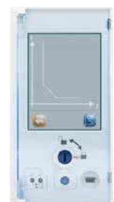
Earth fault tripping curve preview
