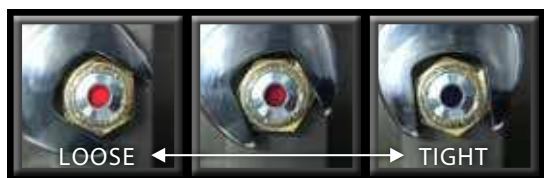
DTI (Direct Tension Indicating) SmartBolts are specialty fasteners with a built-in indicator that shows the tension that has been achieved as the bolt is installed.
